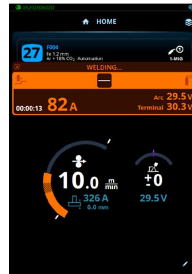
View the welding values and adjust the parameters while the robot is welding.
