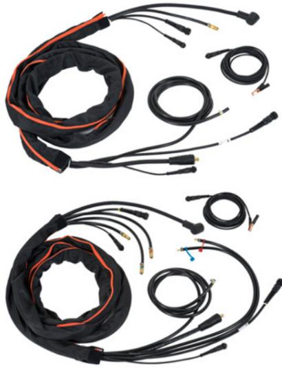
The interconnection cable set contains several cables and hoses. The cable set is used for delivering the welding power, shielding gas, cooling liquid, and control signals from the welding power source to the wire feeder.
