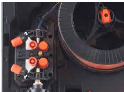
Kempact 253/323 models feature the Dura-Torque four roll wire drive unit.
